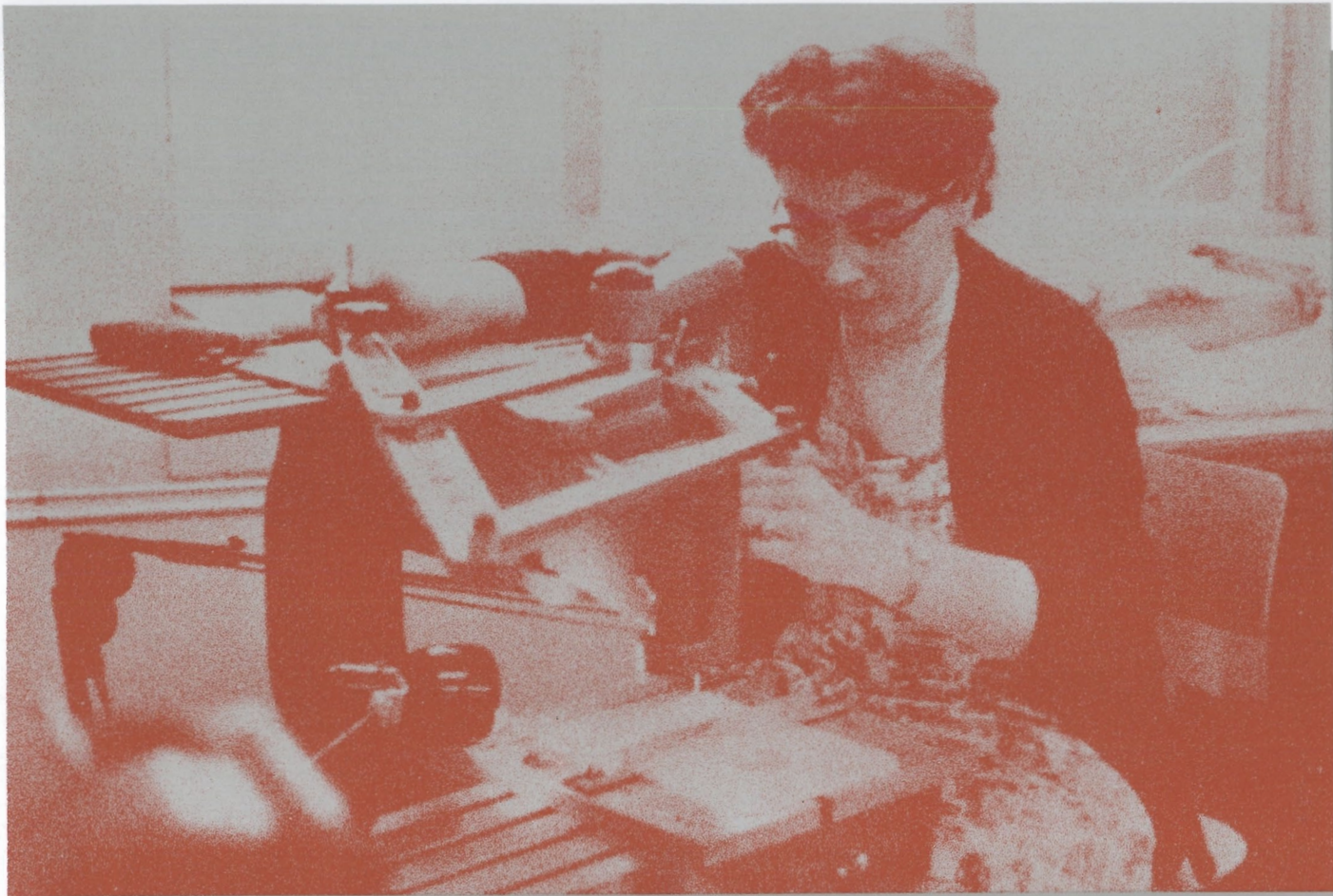
This engraving machine was used by workers at HP Germany to put product numbers and the company logo on instrument panels.
